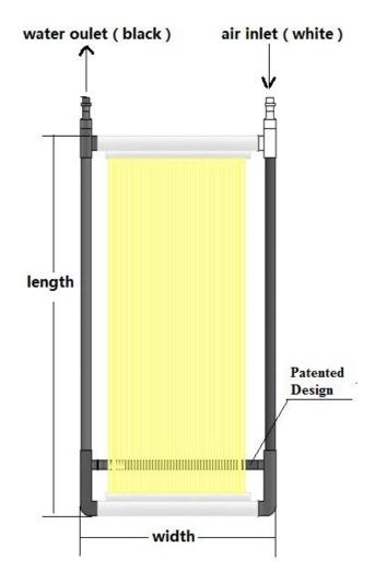
Every module has a separated Multi-pole for air blowing. It can ensure the effect of the air bubble washing the membrane surface.
